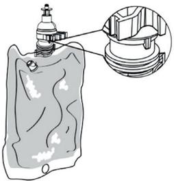
SCREW THE PUMP ON TIGHTLY, ENSURING THE CLAMPS SNAP ONTO THE SOAP BAG EDGE.
