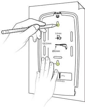
MARK THE POSITION TO DRILL WALL MOUNTING HOLES.
