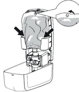
ATTACH THE POUCH WITH THE LABEL FACING THE BACK WALL TO THE HOOK AND VERIFY THAT IT FITS PROPERLY.
