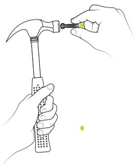
TAP ANCHORS INTO EACH DRILLED HOLE.
