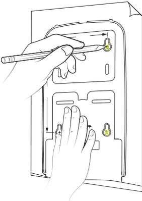
MARK THE POSITION TO DRILL WALL MOUNTING HOLES.
